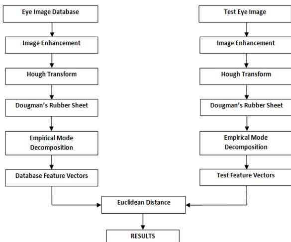
**Fig 2:** Block diagram of IREMD
